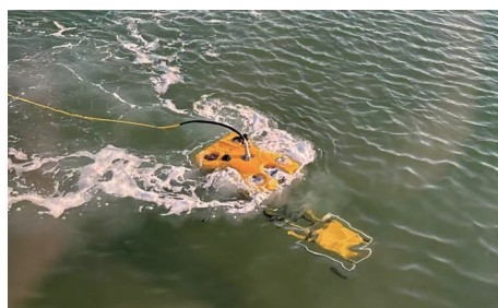
图4 潜载频率域电磁探测系统 Fig. 4 Submarine frequency-domain electromagnetic detection system
